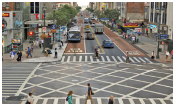
52-foot section: four travel lanes with "bulb out" section for bus boarding and fifth-lane loading zone to the left rear of the standing bus.
