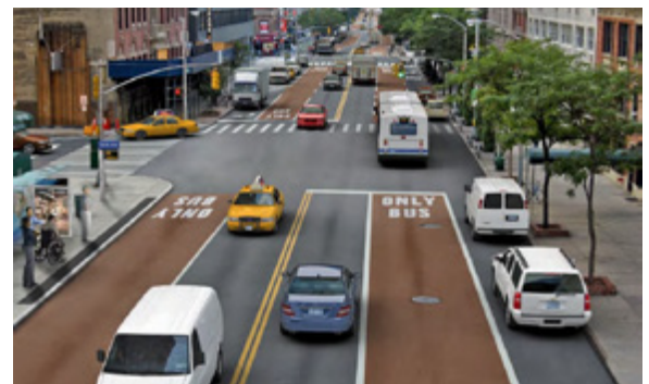
60-foot section: five travel lanes with no loading zone.
